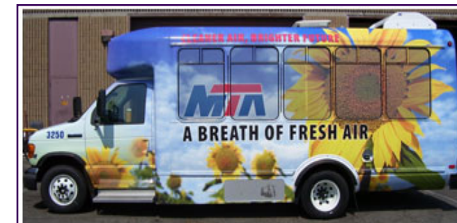
One of the five Flint MTA mini-buses that are retro-fitted with a hybrid electric/diesel system. Plans are to bring hydrogen fuel cell technologies to MTA buses in the city within three years.
